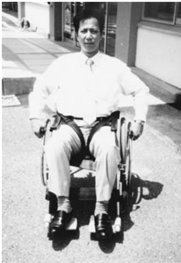
FIG. 3—When the belt is fastened, the belt passes over both sides of the user's abdominal wall nearly at the level of the umbilicus.
