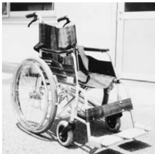
FIG. 2—The right arm of the wheelchair is deformed.
