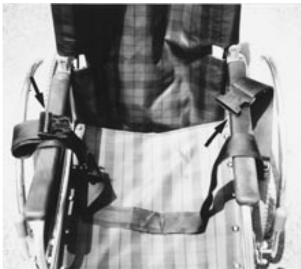
FIG. 1—Wheelchair user restraint system. The center of the belt was stitched to the seat, but some of the threads have been broken. The arrows indicate the location of the buckle that is fastened behind the back of the chair.
